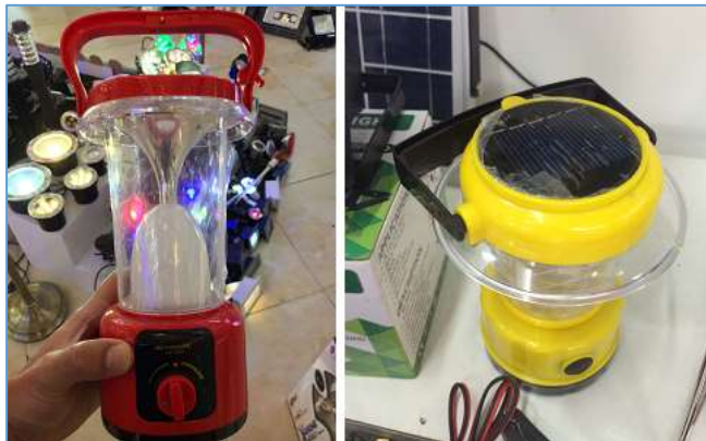
Lights with attached solar cells (0.7 W)
