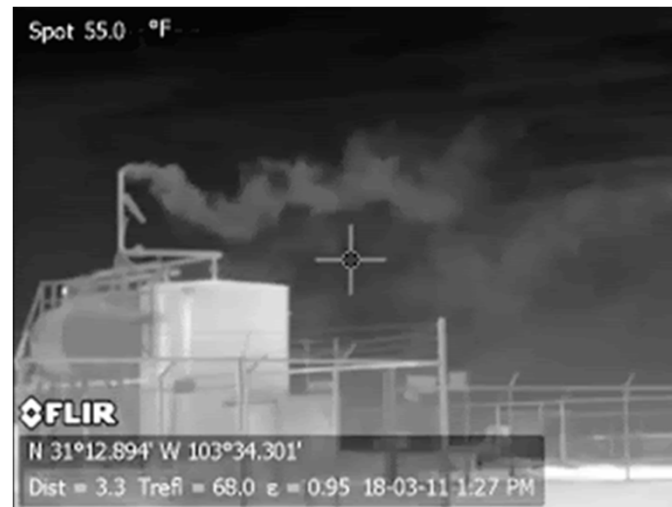
Venting from the tank vent at Energy Transfer Hoban Gin Compressor Station
